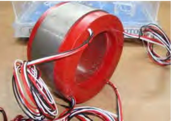
In 2010, Sona College of Technology developed a Slot-less, Brushless DC Electric Motor, called 'MADRAS' (Microwave Analysis Detection of Rain and Atmospheric Structures) and it was incorporated in a space satellite of ISRO.
